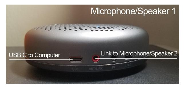
[2] Connect the second microphone/speaker to the first microphone/speaker via the **OUT/LINK** connection on each speaker with the provided aux cable. [3] Connect the included power supply to the USB port on the second microphone/speaker.
